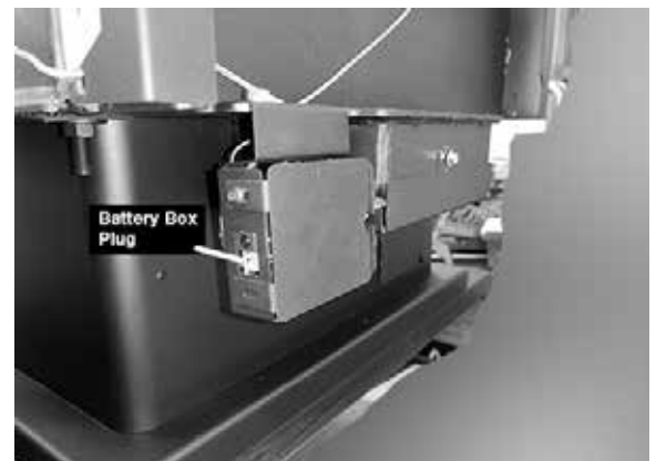
Figure 12. Battery Box plug.
