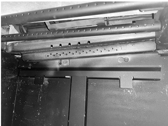
Figure 4. Remove rear baffle
