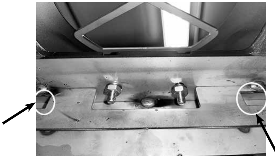
Figure 6. Front mounting slots for Flue Gas Agitator
